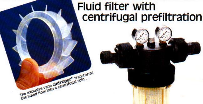
The centrifugal force given to the liquid flow separates the 'larger' particles by throwing them down into the lower bowl. The smaller particles are retained by the filtersleeve, according to the micron-size filter-sleeve chosen.
